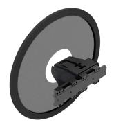
The hatch panel mechanism was designed to slide and pivot any way it needed too in order to passively grab a hatch panel from the human player station. The mechanism has an embedded sensor that uses two LED's and a photosensitive resistor to detect when it has hatch panels in it's possession. When it comes time to let the hatch panel go this mechanism uses a single-acting pneumatic cylinder to release and score the hatch panel. I did the design work for this mechanism and it's embedded sensor.
