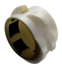
That Fancy geometry came in the form of these wheels with thread shaped scoops. The threads allow the drone to screw into the rocket body keeping the rover secure during flight. These wheels can then spin relative to the rocket body as the main body of the rover is keyed to the thread preventing it from spinning. To test this a wheel and small portion of thread was 3D printed. It was successful in testing so this design has lots of merit.
