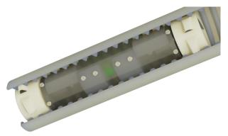
This rover was designed as a part of Pitt's 2019-2020 USLI payload. It was tasked with surviving a rocket flight then collecting an ice simulant made of Injection molding pellets.
